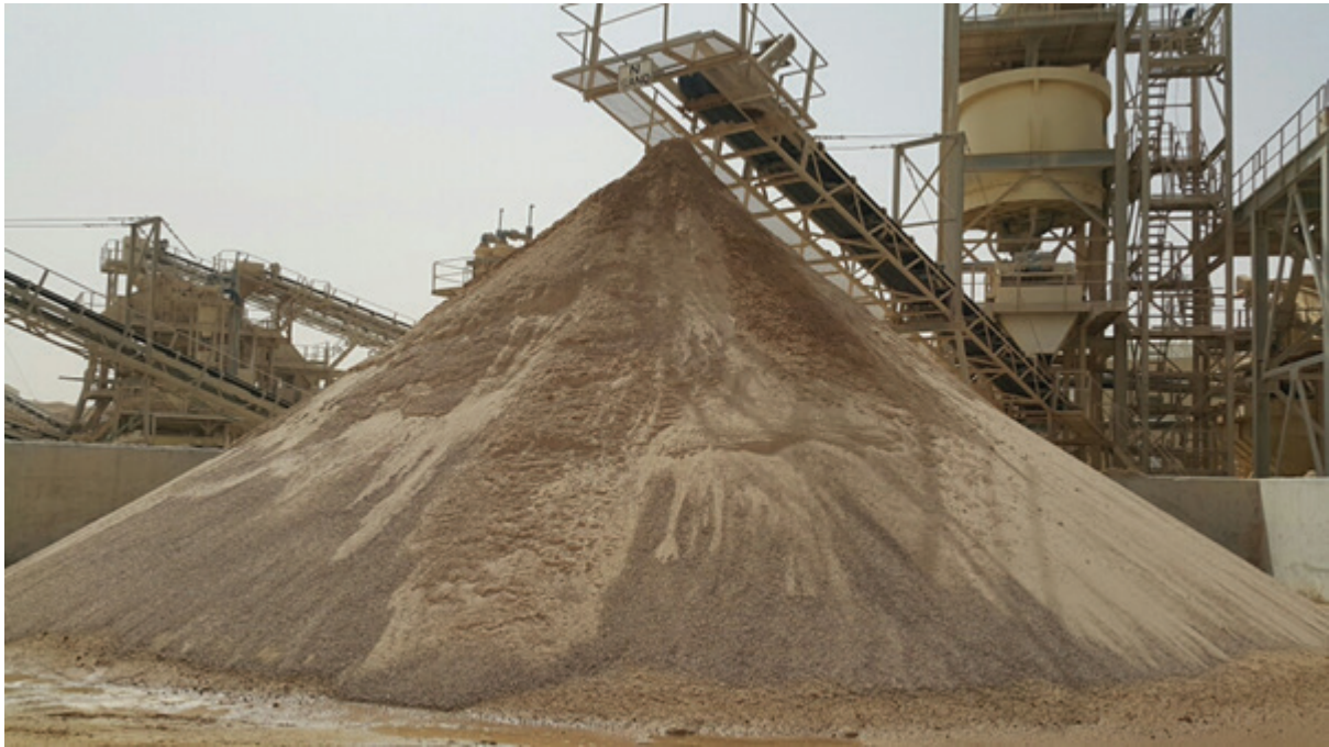
Figure 8-2 Production of washed concrete sand in Qatar
