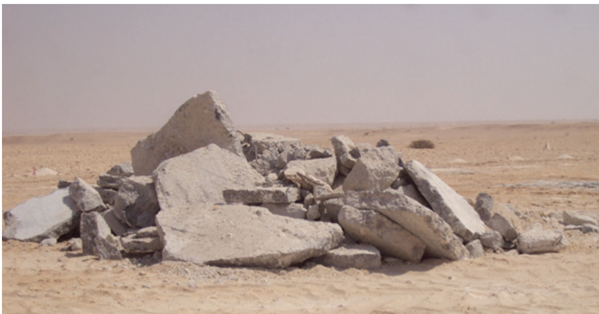
Figure 3-7 Recycled concrete is a clean source of RCA
