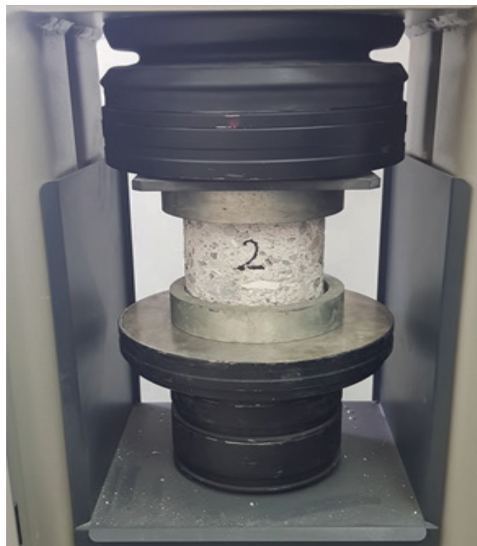
Figure 6-6 Compressive strength testing of the RCA subbase core
