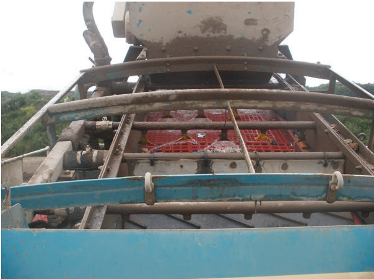
Figure 8-3 Water used for washing of recycled aggregate
