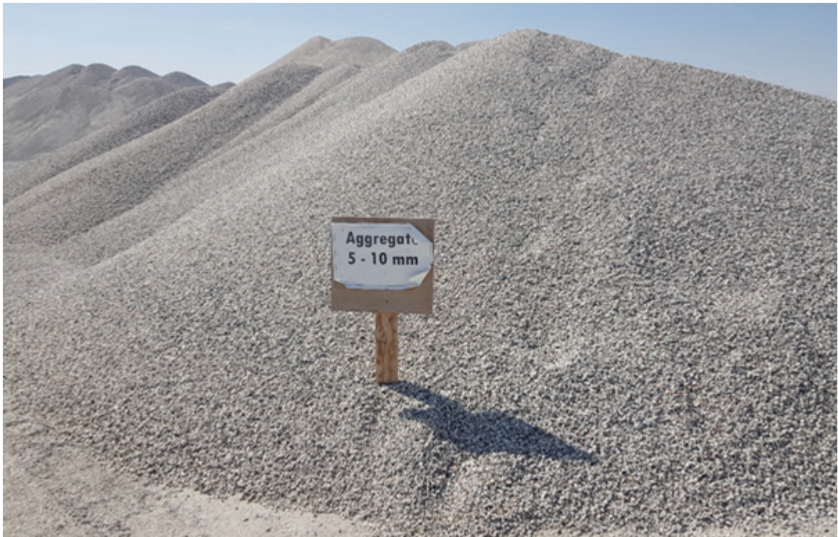
Figure 3-4 EW of 5-10 mm for use in concrete blocks and pipe bedding
