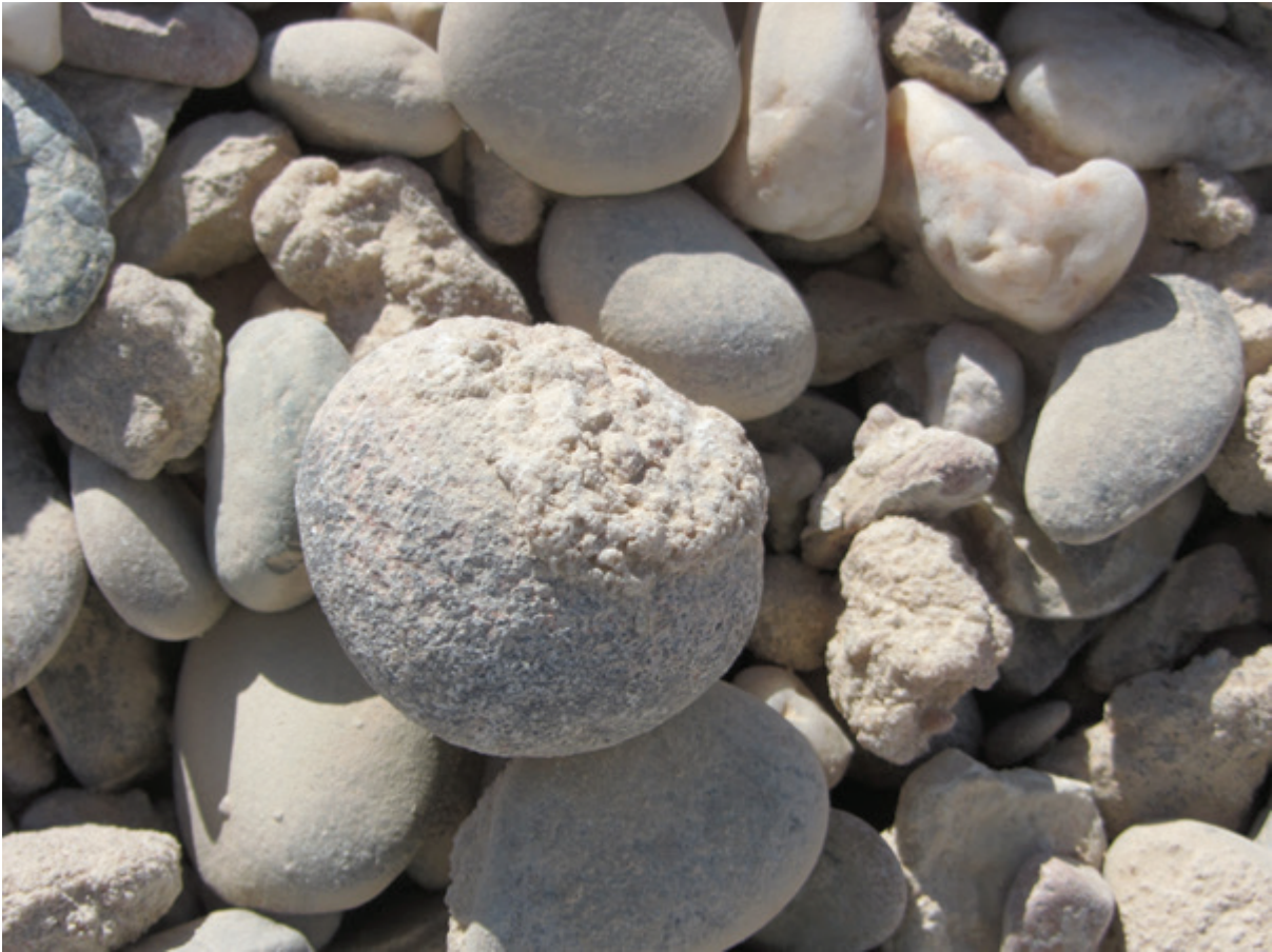
Figure 3-12 Unprocessed Wadi gravel; the sandy lumps are gypsum-bound deposits (GBD)
