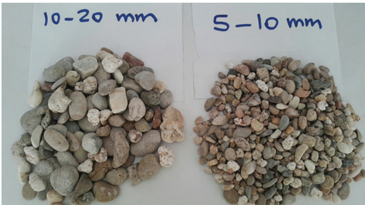
Figure 3-13 Processed Wadi gravel; GBD almost completely removed
