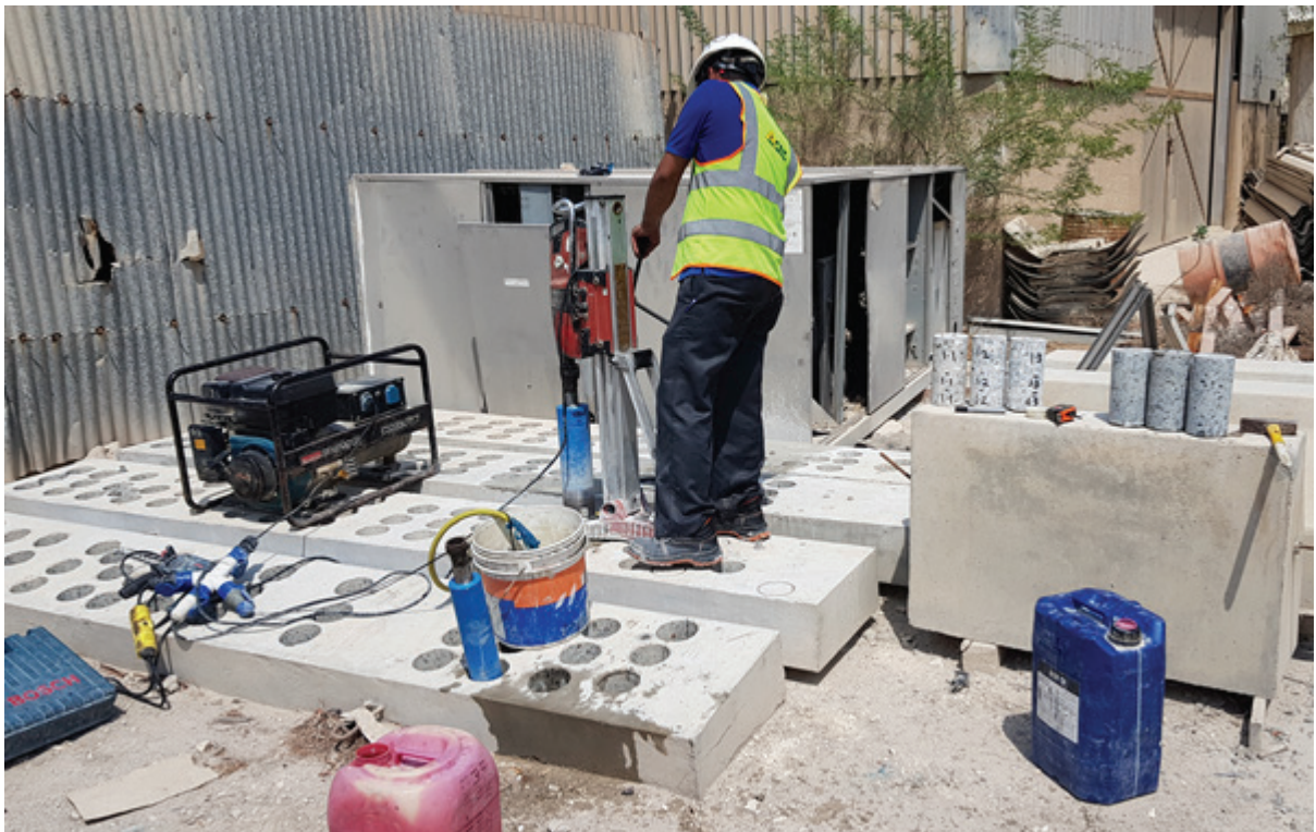
Figure 5-4 Coring of the testing beams at 5 years
