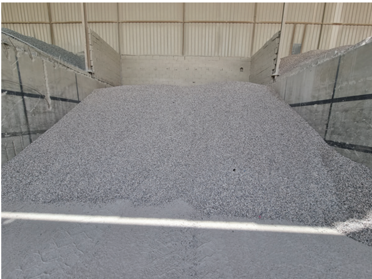
Figure 5-20 Mixed CDW used for the production of concrete blocks
