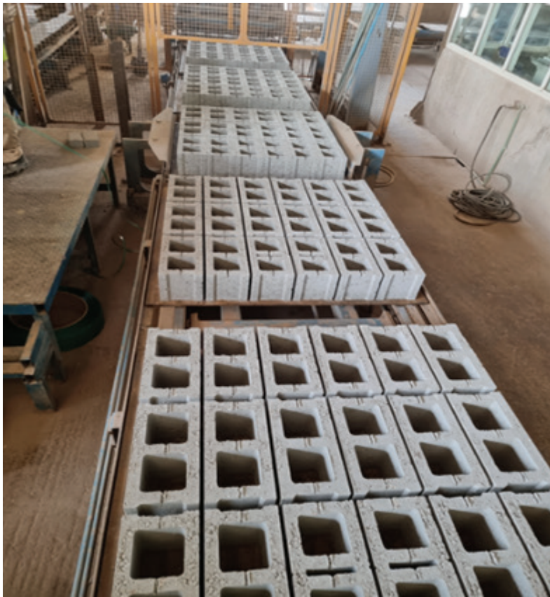
Figure 5-21 Production of concrete blocks with recycled aggregate
