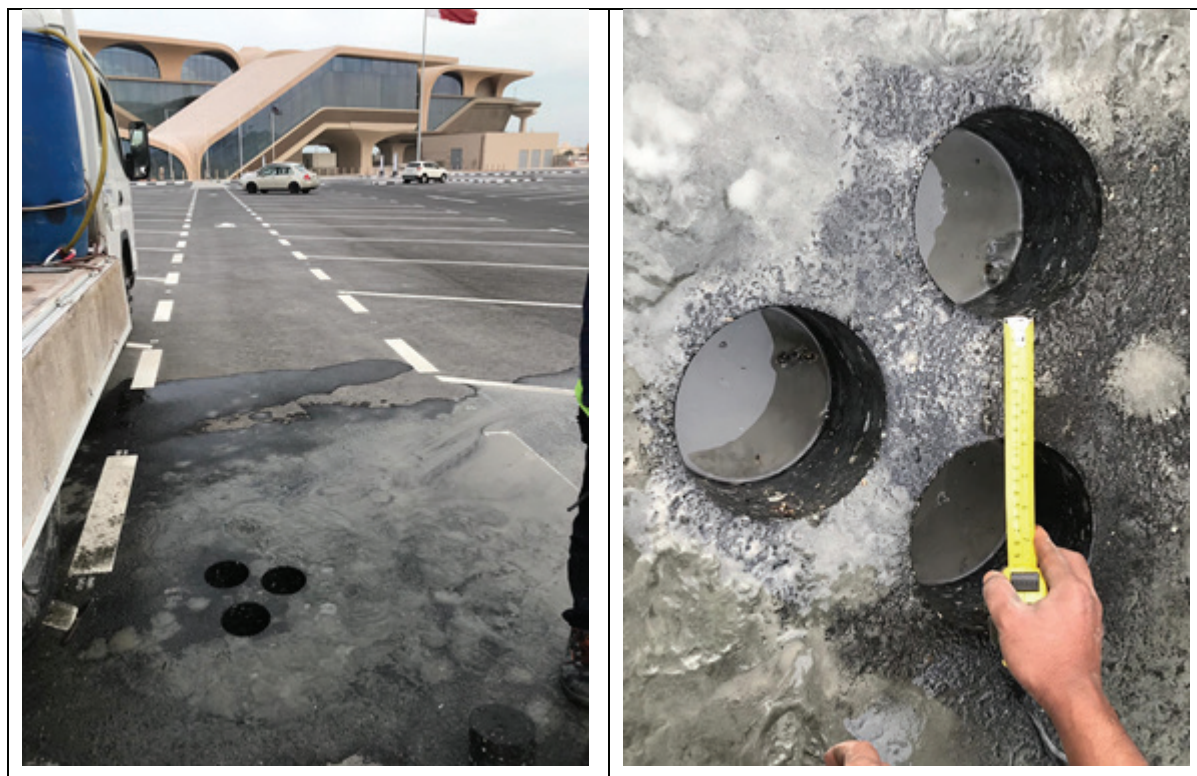
Figure 4-3 Coring of RAP asphalt at a single location– Al-Wakrah Metro car park
