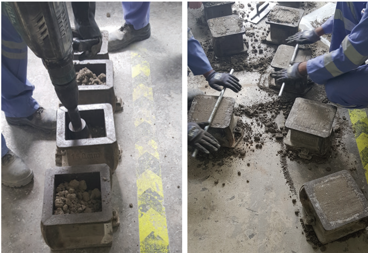
Figure 6-10 CBM compaction (left) and surface levelling (right)
