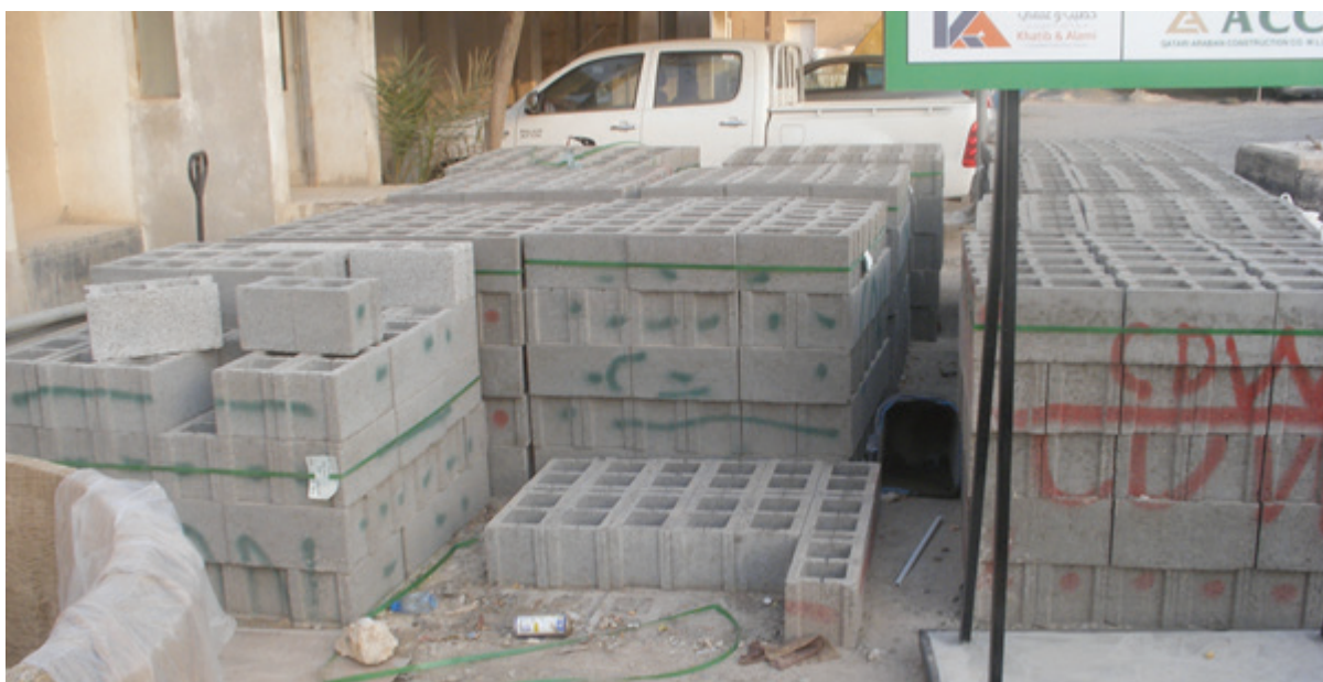
Figure 5-17 Concrete blocks with recycled materials used for testing
