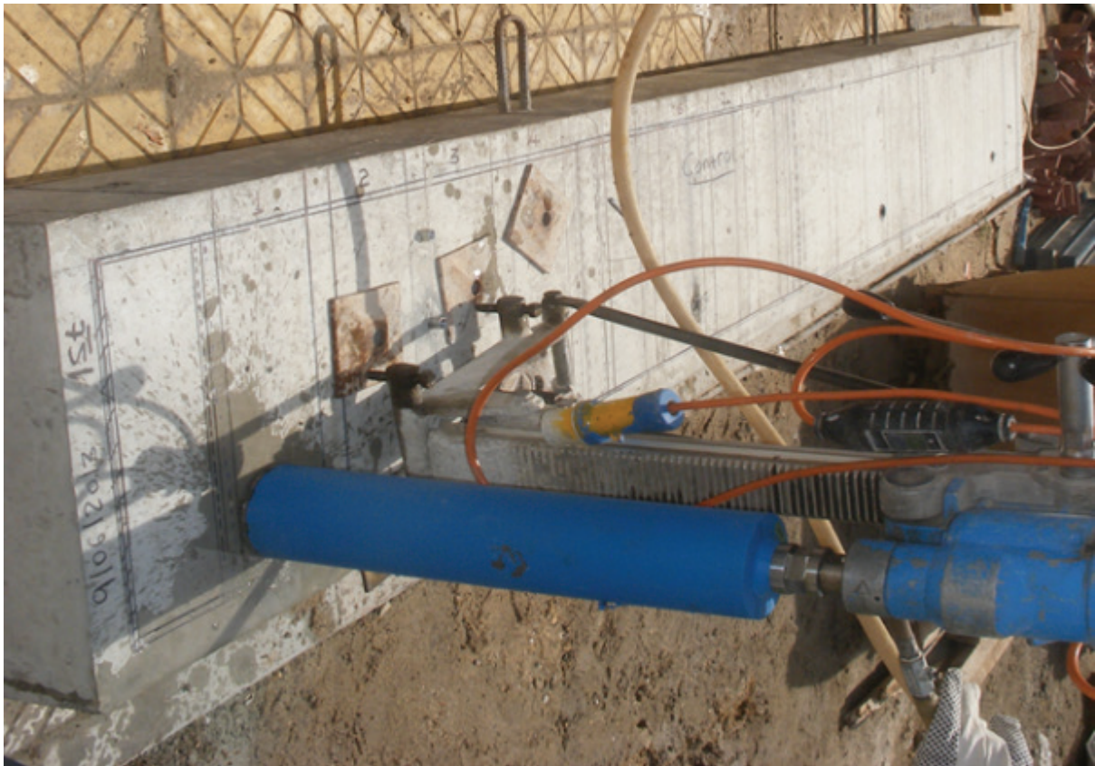
Figure 5-3 Testing beam with marks and initial coring at 28 days
